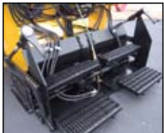
Full featured, heavy duty screed – vibratory, crown/invert, and propane heat.
