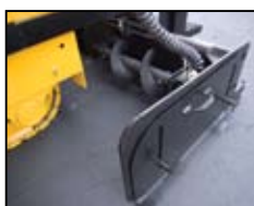
Material sensors keep asphalt delivered to the full width of the screed at all times – automatically.
